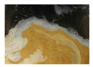
Biofilm removal during the treatment of a balance tank, producing a slimy deposit. Biofilms can protect pathogenic bacteria such as P.Aeruginosa and Legionella against chlorine disinfection.
