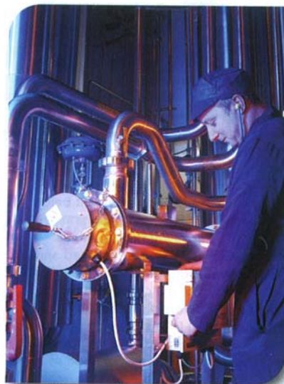
ABOVE: UV arc tubes like this from Hanovia are used also in a range of processes where water passes through the chamber and the UV kills any microorganisms present by disrupting DNA
